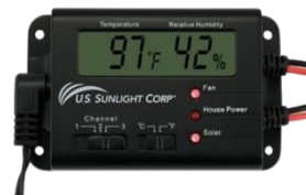
Solar/AC Attic Fan Control
